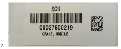
Figure 6-2 Acceptable Formats for Producing Identification Labels. A properly configured identification label will contain required IUID and DPAS Unique Item Identifications (UIIs), nomenclature, serial number and asset ID (12 digits in length).
